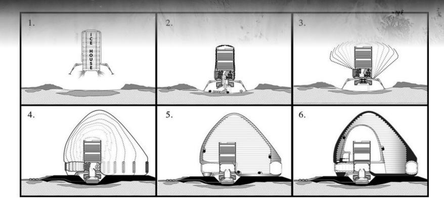
The Mars Ice House Project proposed an inflatable translucent material brought from Earth to be pressurised and filled with ice. Along with the proposed construction technique, the design team also proposed alternative ways to harvest the ice from the soil. Due to the low atmospheric pressure on Mars, the ice sublimates when brought to the surface, and therefore could be harvested as water vapour, which is also partially purifies it.
