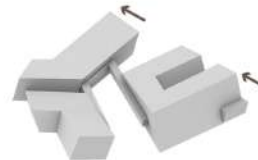
9. North Facades are Leaned Backwards and South Facades are Leaned Forwards for Controlling Sunlight
