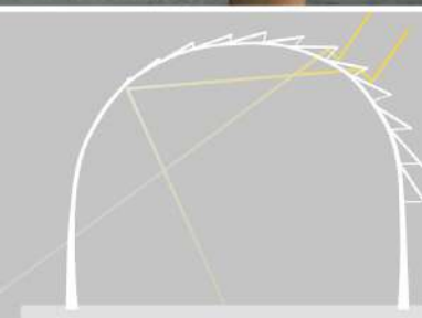
The pavilion is designed to allow indirect sunlight from south with gradually displaced shading elements
