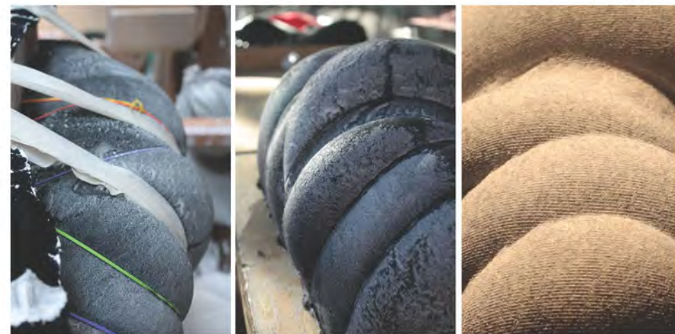
Test 4 This step scrapped the modular framework for experimenting with how the formwork (merely fabric, rubber bands, and masking tape) could be manipulated during the casting process to obtain a desired cast form.
