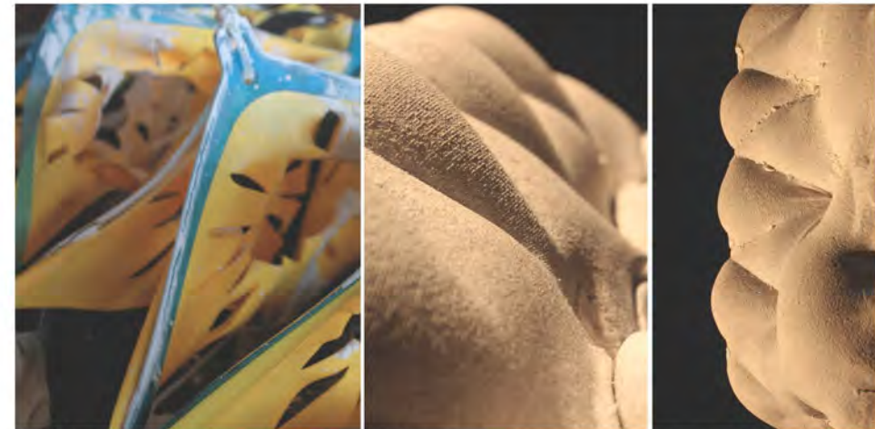
Test 6 Initial modules are rearranged to form a larger system. In this particular iteration the fabric utilized as a secondary control device stretches too much and thus doesn't articulate the surface texture in previous iterations.
