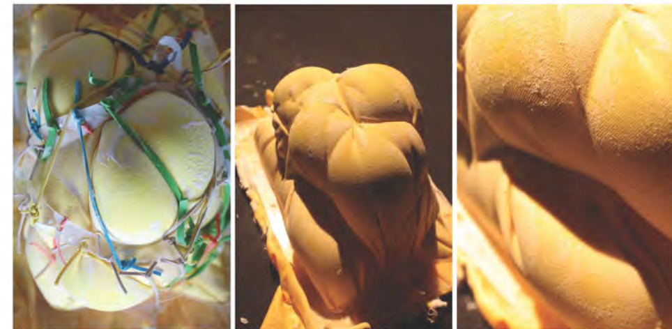
Test 5 This step alters the module to have a higher number of connection points where the tensile structure (rubber bands) can intersect each frame. Tensile members of different thicknesses/force-exerting capacity are introduced uniformly and the cast form 'accidentally' expresses an aesthetic of incremental controls.
