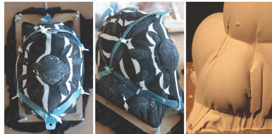
Test 3 This step takes away the number of frames and allows the patterned, less stretchy fabric to perform as a constraining device. Cast result portrays secondary extrusion textures as a result of this controlled system of incremental-bulbosity.
