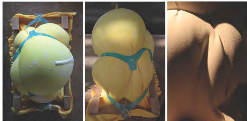
Test 1 Initial system of (1) malleable frame, (2) tensile supporting structure, and (3) fabric membrane. Gravity informed bulbous extrusions. Fabric provided cast piece with stress lines as evidence of the restraint on the form provided by a finite piece of fabric.
