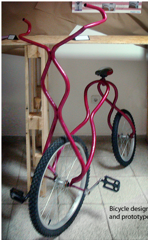
Design of a bicycle, using welded steel tubes and bicycle tires, 2010
