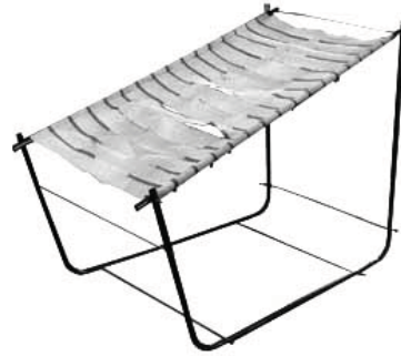
prototype 1_ unstable frame / not enough tensile support for elastic
