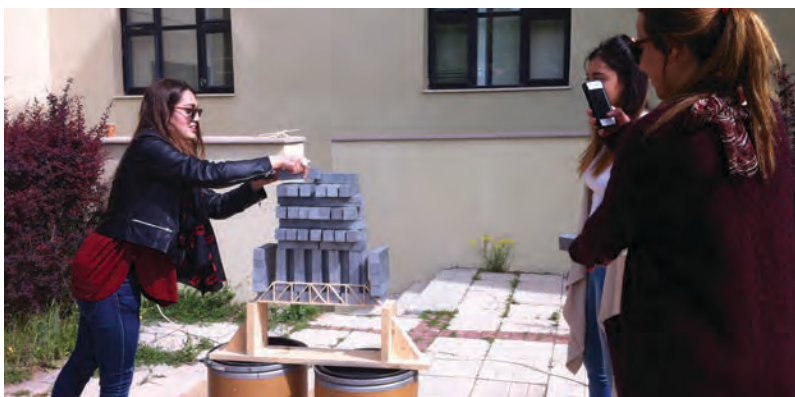
Pelin Sokmen, Iris Gul, İrem Ceri, Load Carried: 122 kg, Bridge Weight: 105 gr, an alltime record, ARCH231, Spring'14.
